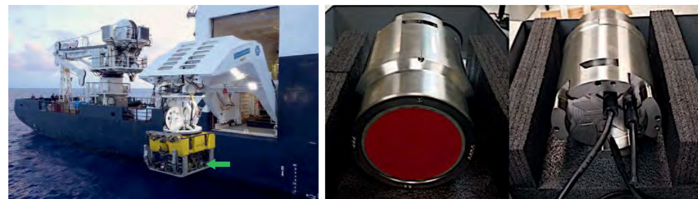
Left: Figure 4. The custom-made BXL-79 remotely operated vehicle being deployed from the research vessel Petrel . The green arrow in the picture shows the location of the Teledyne RDI Pioneer-300 Doppler velocity log. Photo courtesy of Paul G. Allen. Right: Figure 5. The Teledyne RDI Pioneer-300, the first Phased Array DVL rated to a depth of 6000 metres
