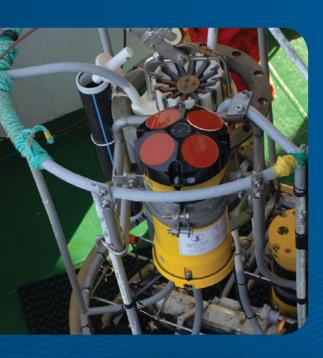
Teledyne RDI ADCP mounted on a hydrographic rosette, ready to be lowered to the seabed.
