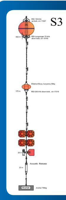
Mooring Design. At S3, three Teledyne RDI ADCPs were installed, using top and mid-water buoys.
