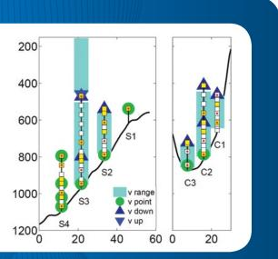
Mooring layout at Slope (S) and Channel (C) sections. ADCPs: blue triangles. Depth (m); distance (km).
