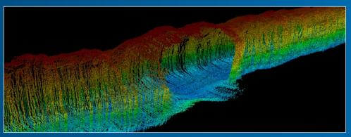
3D profile data image showing the solid integrity of the tunnel
