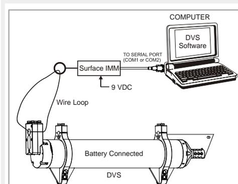
Loop a conductor through the DVS inductive modem and the surface inductive modem (not supplied) connected to a computer.
