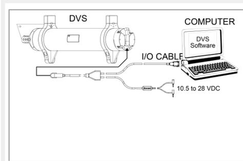
Remove the dummy plug from the end-cap and connect the I/O cable to the DVS end-cap.
