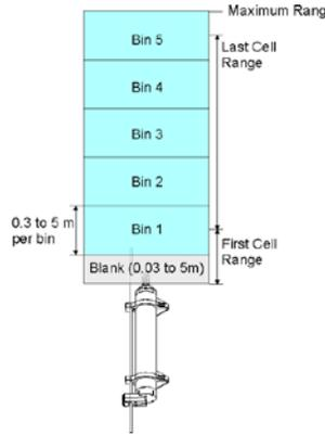
**First Cell Range** – The range from the transducer face to the middle of the first depth cell (bin). The depth cell (bin) size and the WF (blank) command in the command file primarily affect where it is located.
