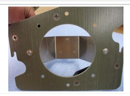
Install the stainless bracket to the instrument mounting plate using the  $^{1}\!/_{4}$ -20 x 5/8" screws, flat washers, and lock
