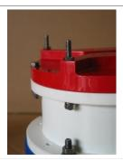
With the ADCP looking downward, sitting on its cap, install the ½-20 x 3" mounting studs. Insert the stud from above and install a lock washer and standard nut on the bottom, leaving no more thread than necessary protruding from the bottom of the nut.
