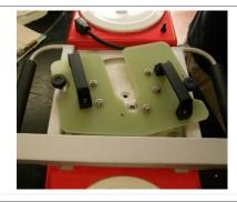
Place the instrument assembly into the main hull. Rotate clockwise and tighten the thumb turns.
