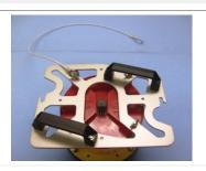
The safety cable provides a vital link from the ADCP to the tow line. Use the eye nut at one end of the safety cable to secure one of the forward ADCP mounting studs to the instrument plate.
