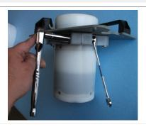
Slide the instrument plate, with clamp attached, over the top side of the M9. Tighten the clamp to lock the instrument in place.
