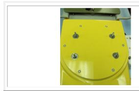
Slide the electronics box with base plate over the mounting studs.
