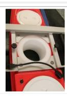
Place foam plug into center of Main Hull.
