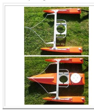
Attach the Wire Rope Bridle to the crossbar by turning the U-bolt connector screw counter-clockwise. Firmly tighten the connector screw onto the crossbar bridle by turning bolt in a clockwise direction. (See figure 4.1 and 4.2)
