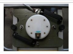
Slide the M9 Instrument Assembly into the hull with the impulse connector facing the rear right corner of the boat. Turn the M9 Instrument Assembly clockwise to engage the locking studs and then tighten the thumb-turns to secure the assembly.
