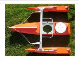
Attach the Main Hull to the Crossbar using the  $\frac{1}{4}$ -20 x 1" screws with  $\frac{1}{4}$ " lock washers and  $\frac{1}{4}$ " flat washers provided.
