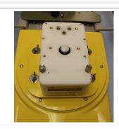
Secure electronics box assembly with lock washers and wing nuts.
