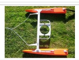
Attach the Outriggers to the crossbar using the ½-20 x 1 ¾ socket head screws with ¼ lock and ¼ flat washers.
