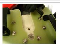
With the ADCP looking downward, sitting on its cap, align instrument plate holes to the holes on the RiverRay instrument.
