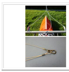
Attach the other end of the safety cable to the carabineer on the Wire Rope Bridal as shown.
