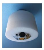
Begin by placing the foam seal ring around the instrument with only the sensors protruding, as shown.
