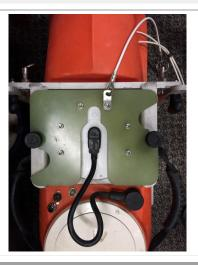
Install the instrument by laying the mounting plate over the thumb turns and turning it snugly into place. Tighten the thumb screws to secure.
