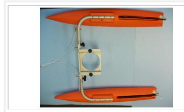
Next, attach the outriggers to the crossbar using the M6 x 35mm oval head screws provided.
