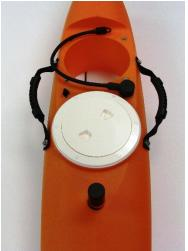
The 12v 7.2 ah SLA battery (provided) powers the instrument and data transmission system, and power to both systems is controlled by the on/off toggle on the deck.
