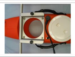
Attach the main hull to the crossbar using the M6 x 16mm pan head screws with lock washer and flat washer as shown.
