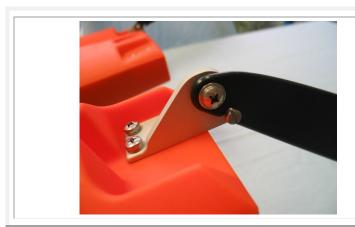
Note that the notch in the fin seats onto the slotted-head shoulder bolt. This prevents the fin from lowering too far into the water. The shoulder bolt is installed with Loctite.
