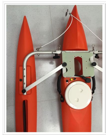
Rotate the brace under the thumb screw on the instrument mounting plate.
