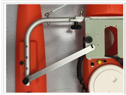
Attach the support brace using the provided thumb screws.
