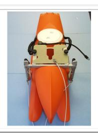
Loosen the folding crossbar two arm knobs before engaging / disengaging the spring plunger assemblies. Fold the Crossbar with outriggers under the Main Hull.
