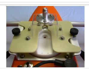
Attach the stainless steel GPS antenna mount to the clear acrylic antenna mounting bracket using the 10-24 x ¾ inch pan head Philips screws, #10 flat washers and 10-24 nylock nuts as shown.
