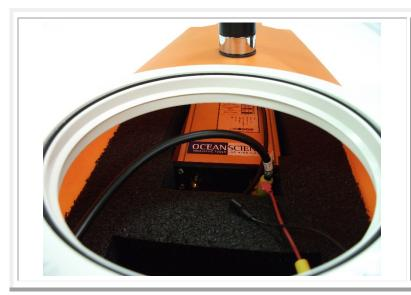
Rotate the modem and slide it horizontally towards the stern (rear) of the boat. The foam liner is cut specifically to fit these modems securely. Make note that the wiring harness or antenna cables are not kinked or stretched. The figure on the left shows the modem in its intended position.
