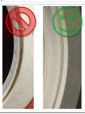
The deck plate O-ring should be cleaned whenever the deck plate is opened and replaced **BEFORE** it is showing any signs of wear and tear.
