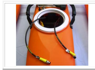
Connect the two internal data cables together to stream GPS data to the RiverRay ADCP.
