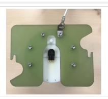
Attach the instrument mounting plate to the ADCP using the M6 socket head cap screws and flat washers as shown.
