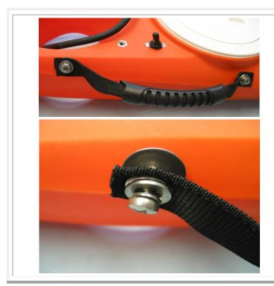
Strap handles attach in this order: hull, fender washer, strap handle, flat washer, lock washer, screw.
