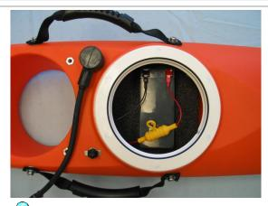
Check the deck plate O-ring each time it is opened.
