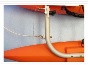
Begin by attaching the wire rope bridle to the crossbar. Insert the Eye Bolt thru each crossbar side as shown. Tighten the nut to 26 IN-LB, 4.0 Nm.
