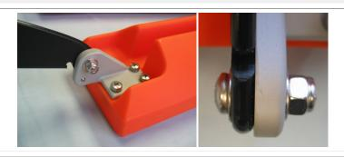
The fin gudgeon attaches using three M6 x 16mm screws with lock washers.
