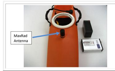
This shows the boat, battery and modem. The MaxRad antenna shown is not standard on a RiverRay boat, unless it is purchased with modems. If your boat does not have a MaxRad antenna, contact Teledyne RD Instruments for instructions on installation.
