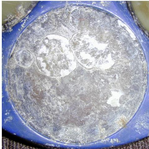
**Figure 15. Barnacle Damage to Urethane Face**
