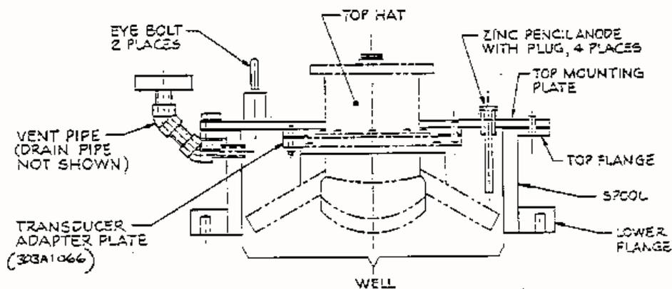
Figure 70. Expanded View of a Sea Chest
