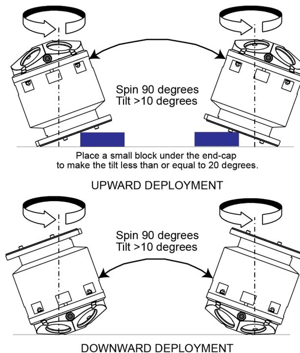
**Figure 30. Compass Calibration**
