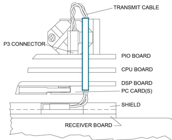
**Figure 43. Transmit Cable**
