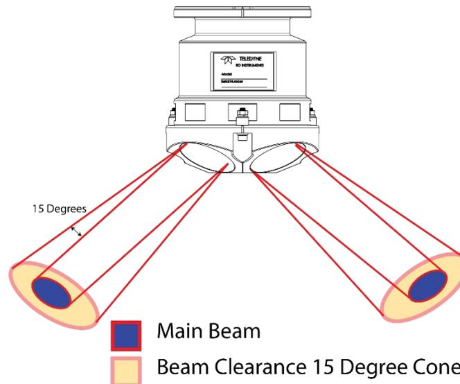
**Figure 13. DVL Main Beam and Clearance 15° Cone**
