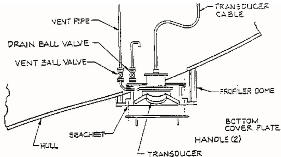
Figure 69. Side View of Transducer and Sea Chest in a Sloping Hull
