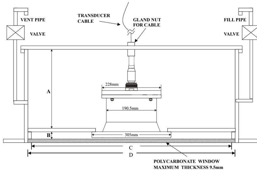
**Figure 96. Underneath Vessel Mounting - OS 150 kHz Flanged Transducer**
