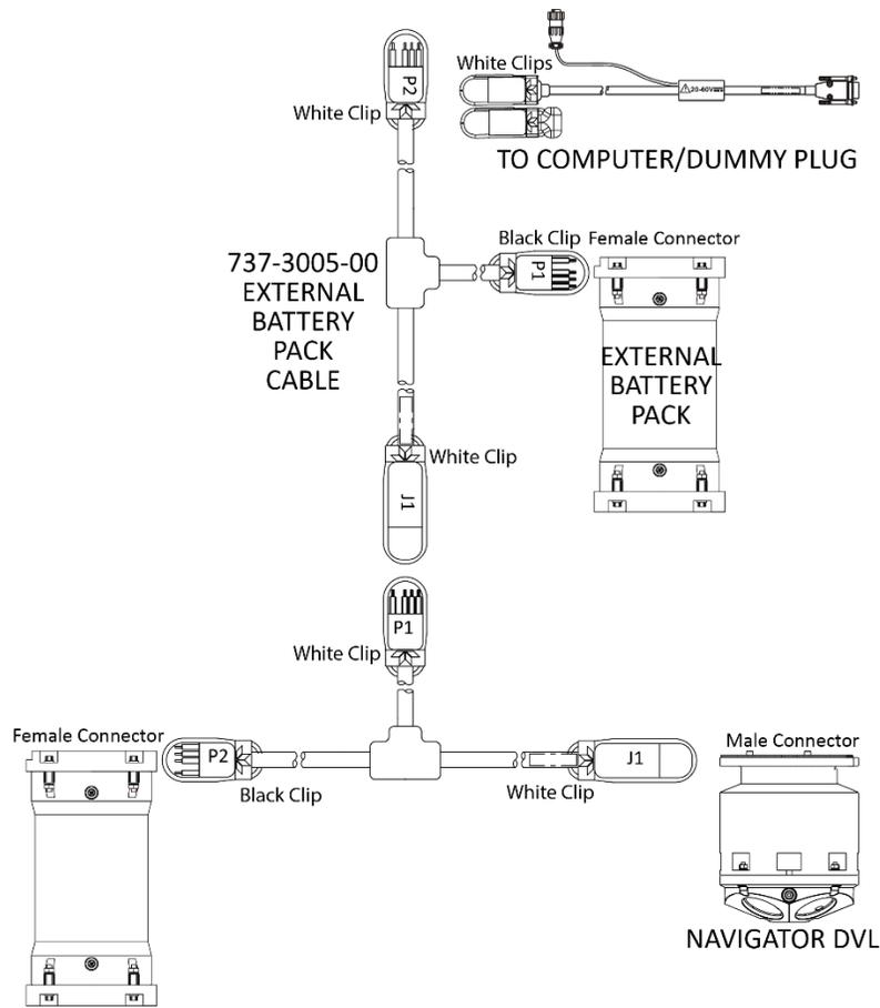
**Figure 4. External Battery Pack Connection**
