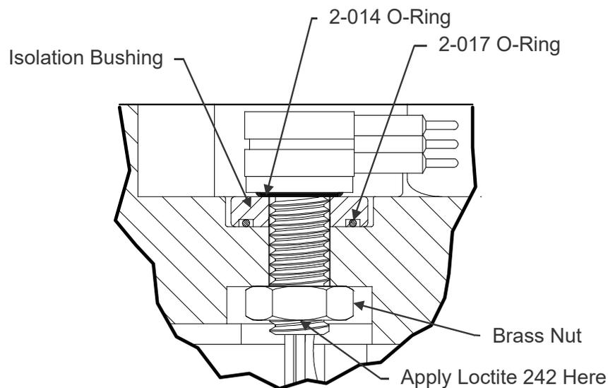
**Figure 37. End-Cap Connector with Isolation Bushing**
