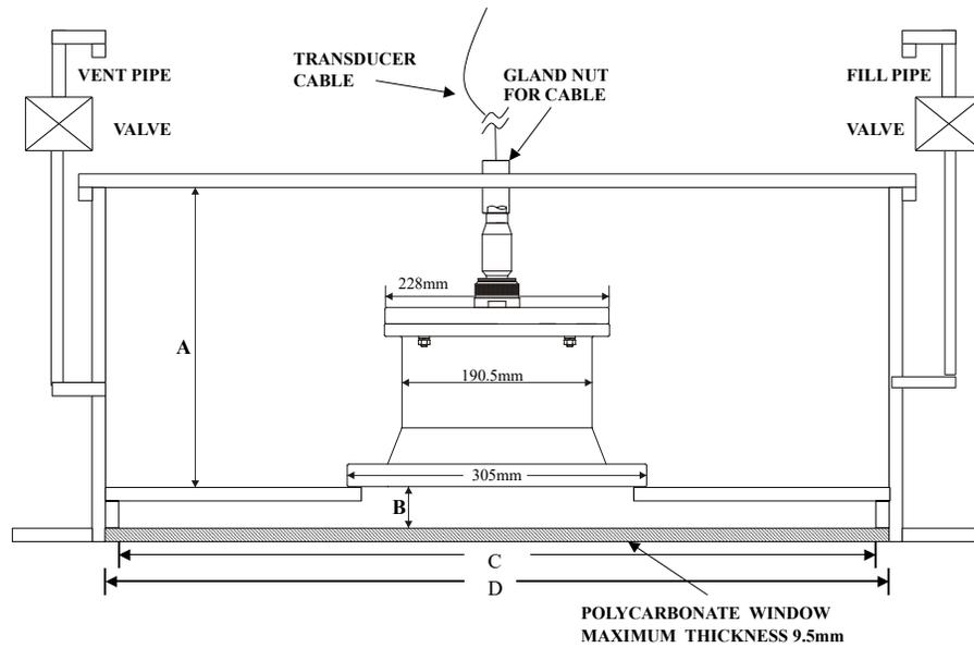
**Figure 95. Inside Vessel Mounting - OS 150 kHz Flanged Transducer**
