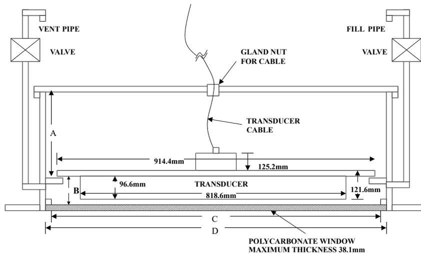
**Figure 91. Inside Vessel Mounting - OS 38 kHz Transducer**
