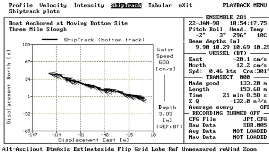
**Figure 74. Ship’s Track showing Bottom Track Bias**
