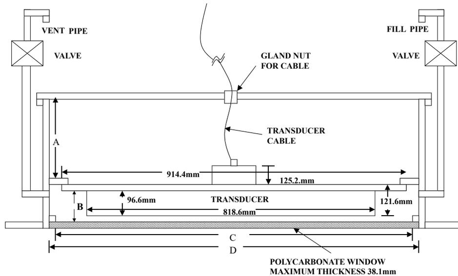
**Figure 92. Underneath Vessel Mounting - OS 38 kHz Transducer**
