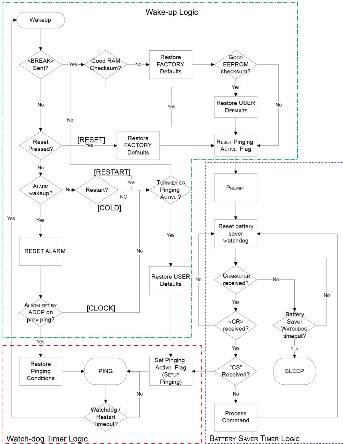
Figure 50. Navigator Wake-up and Timer Logic
