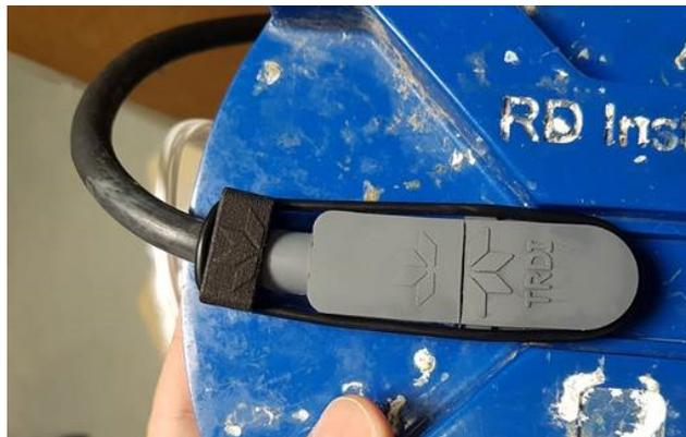
The P2 Plug on the Y cable needs to be connected on the Female connector on the External Battery pack. Use a Black Clip with the long O-ring.
