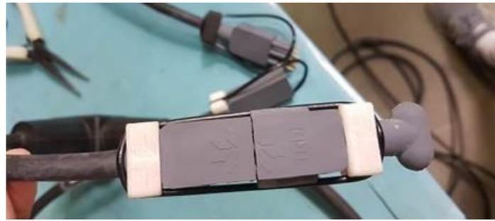
The 3<sup>rd</sup> plug on the Y cable may not be used when there is only one External battery case or when the customer is not using a direct connection with the ADCP. In this case, use the Dummy plug from the ADCP to protect the 3<sup>rd</sup> plug on the Y cable.
