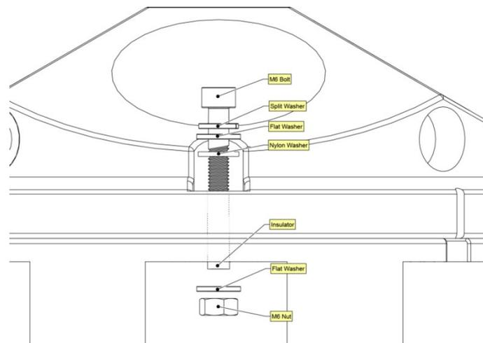
Figure 27. Transducer Mounting Hardware – 1200 kHz
