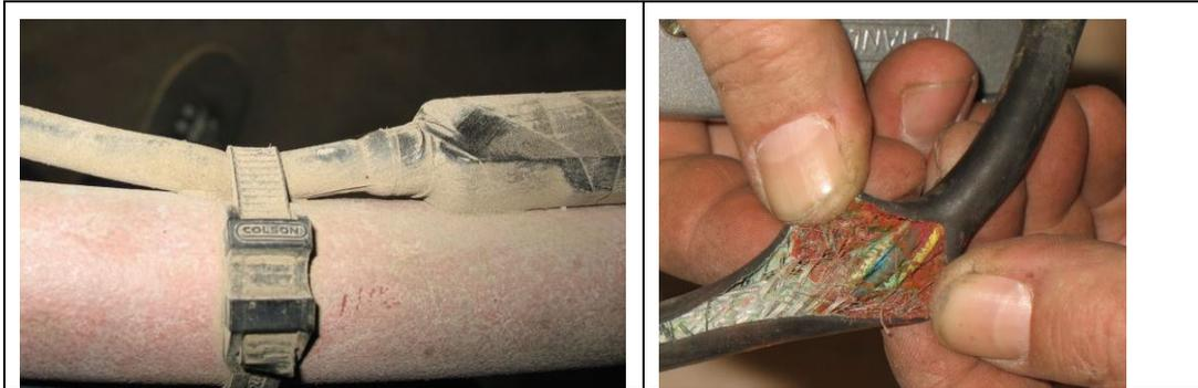
**Figure 5. Do not use Zip-Ties Directly on Cables**
