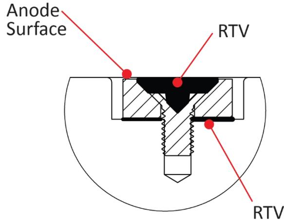
5. Set the new anode in place and tighten the screw to  $1.7 \pm 0.2$  N-M ( $15 \pm 1.5$  IN-LB).
