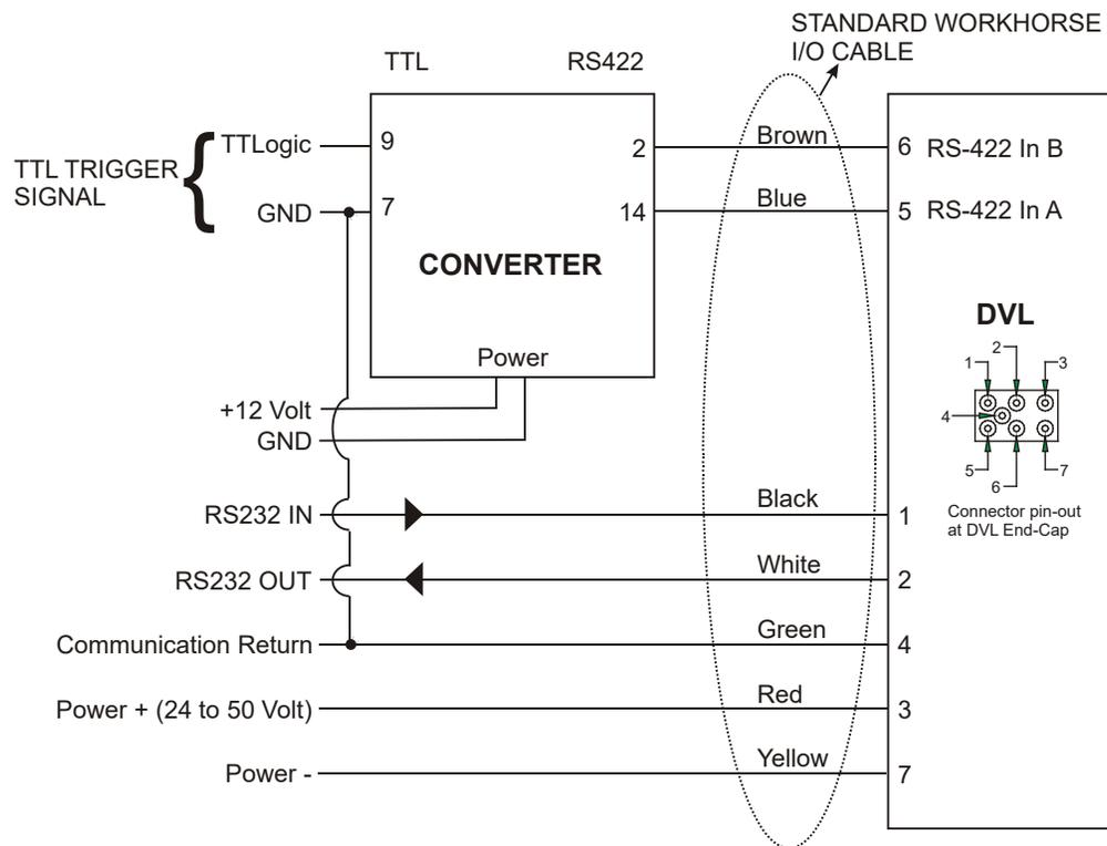
**Figure 99. Triggering a DVL with a TTL Signal**
