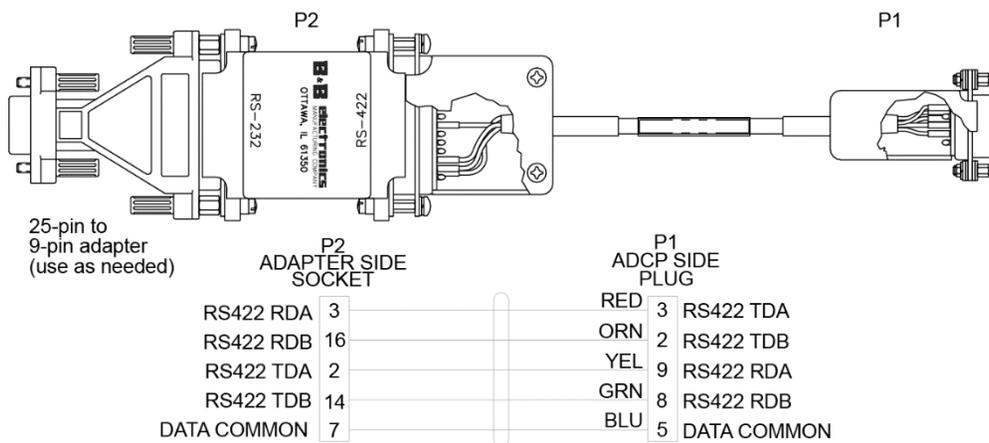
**Figure 49. RS232-to-RS422 Converter Wiring (25-Pin to 9-Pin)**
