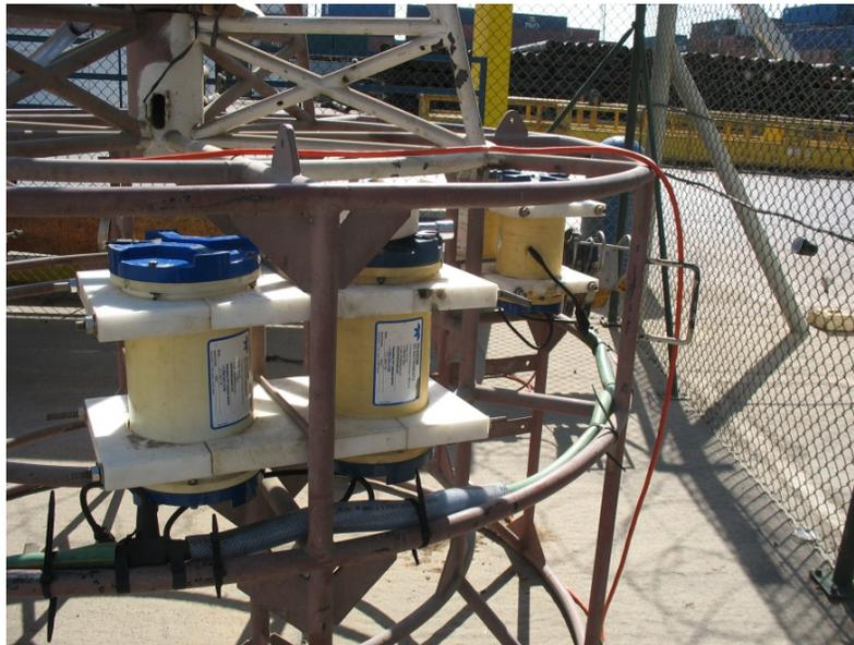
**Figure 6. Cables Protected with Hose**
