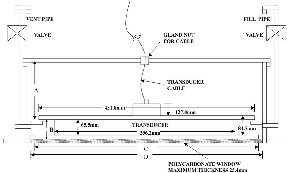
**Figure 93. Inside Vessel Mounting - OS 75 kHz Transducer**
