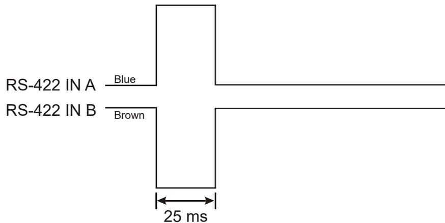
**Figure 100. Timing Pulse**
