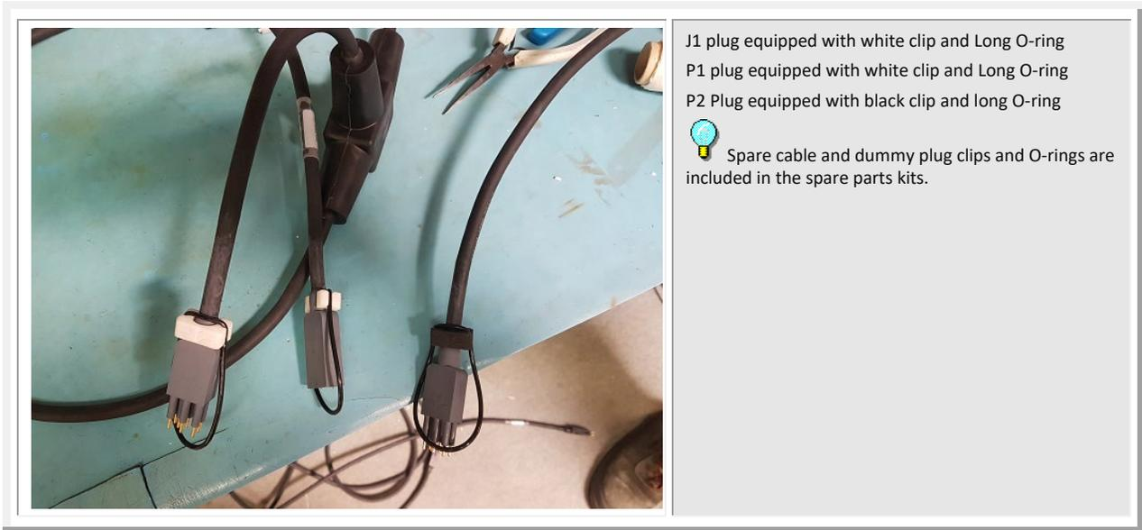
J1 plug equipped with white clip and Long O-ring
