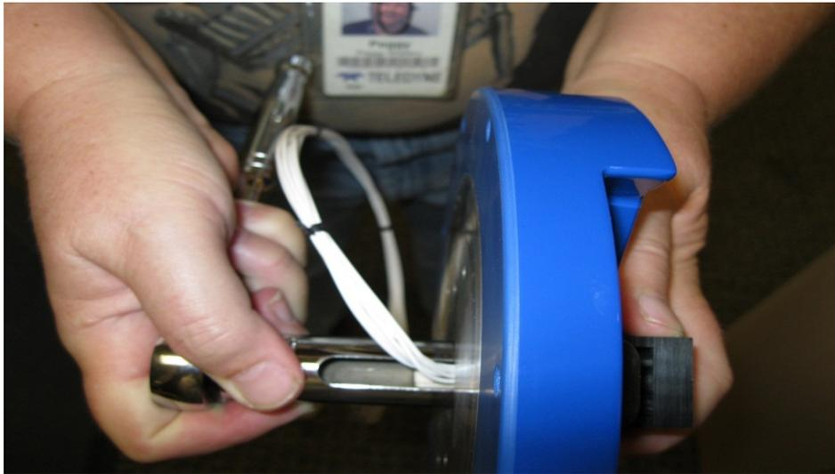
**Figure 36. Removing the Connector**
