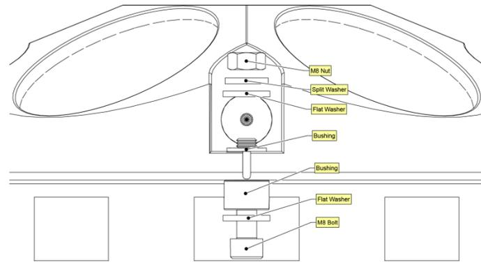
**Figure 28. Transducer Mounting Hardware – 300/600 kHz**
