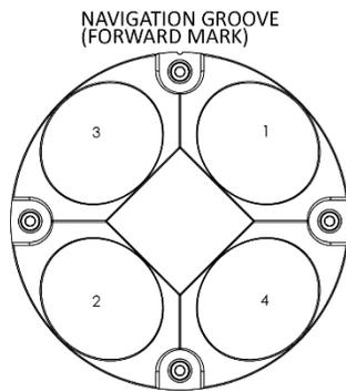
Figure 24. Transducer View
