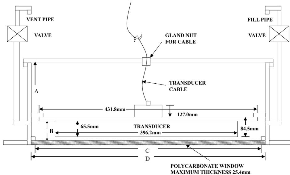
**Figure 94. Underneath Vessel Mounting - OS 75 kHz Transducer**
