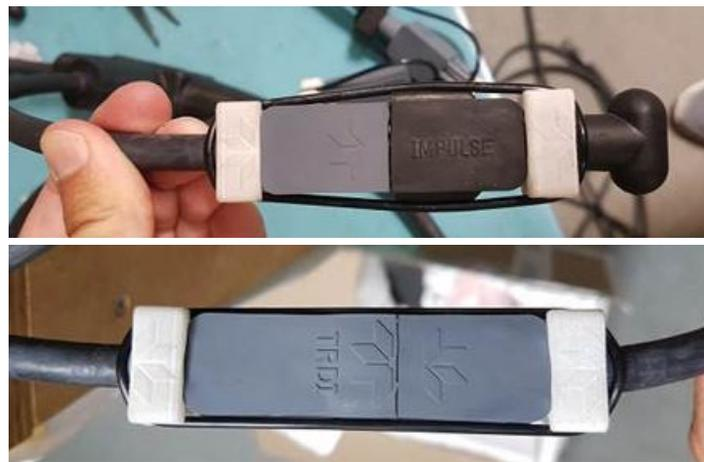
For the P1 plug on the Y Cable 737-3005-00 use two white clip with the long O-ring, This solution works for both the cable connector or for the Dummy plug (New and old design ) when you are not using the 3<sup>rd</sup> Plug on the Y cable.
