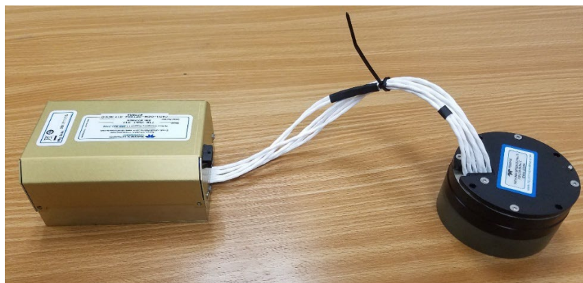
Figure 6. OEM 600kHz Pathfinder Transducer Connections
