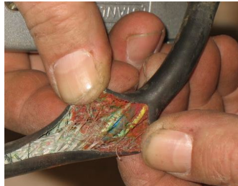
Figure 23. Do not use Zip-Ties Directly on Cables
