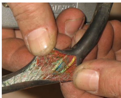
Figure 24. Do not use Zip-Ties Directly on Cables
