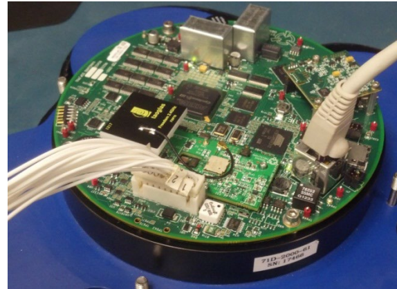
Figure 81. Power I/O Cable Connection
