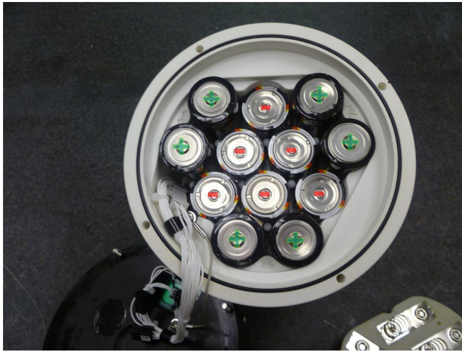
Figure 57. D cell Battery Replacement
