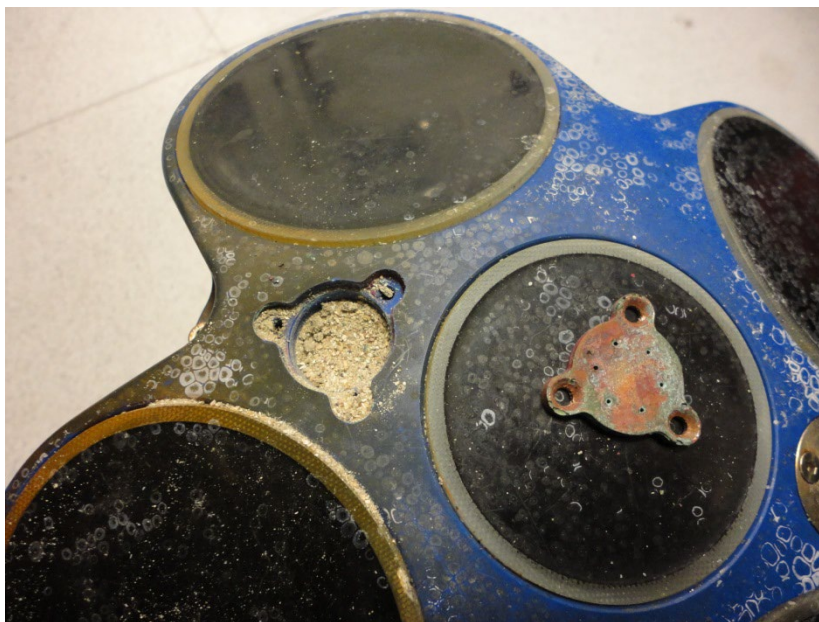
Figure 74. Pressure Sensor Cavity with Sand
