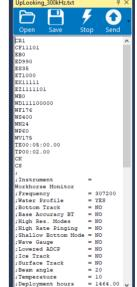
If the system is setup for a delayed deployment, the ADCP sets its alarm clock to the TF command setting, goes to sleep, and waits until time TF before beginning the data collection process. Once pinging, these audible beep and data output indicators will be observable.
