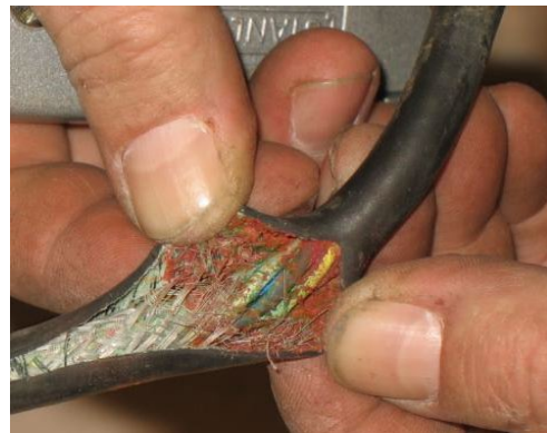
Figure 17. Do not use Zip-Ties Directly on Cables
