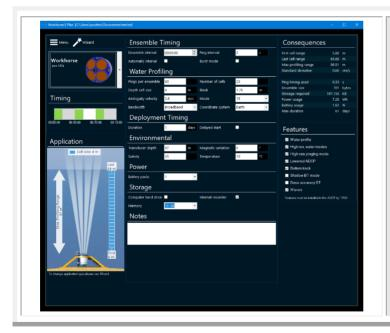
Use the *Workhorse II Plan* software to create a deployment command file for a system with WHII electronics.
