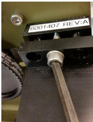
Remove the remaining two longer M6X18mm Hex head screws holding the base and cover to the chassis. Pull back the cover to expose the encoder unit base.
