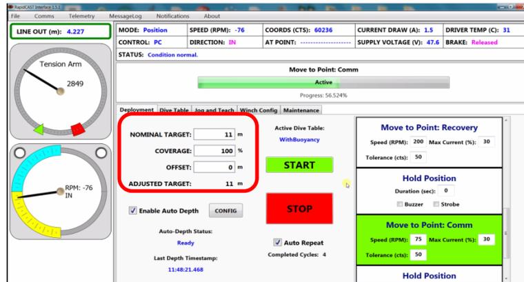
RapidCAST Interface 1.5.1 introduces a multiplier factor called **Coverage**. **Coverage** is a positive-valued parameter that can adjust Nominal Target Depth from 0% thru +100% to give the user increased flexibility in specifying a correction factor. In the context of depth correction, these fields take on the following meaning:
