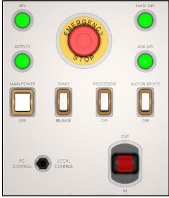
The control panel features several components: a central red 'EMERGENCY STOP' button, four green indicator lights labeled '48V', 'ACTIVITY', 'MAIN 24V', and 'AUX 24V', four toggle switches labeled 'MAIN POWER OFF', 'BRAKE RELEASE', 'PROCESSOR OFF', and 'MOTOR DRIVER OFF', a 'PC CONTROL' port, a 'LOCAL CONTROL' port, and a red 'OUT IN' switch.
