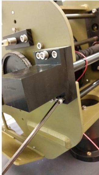
Remove the four recessed Hex head screws holding the encoder cover to the base.
