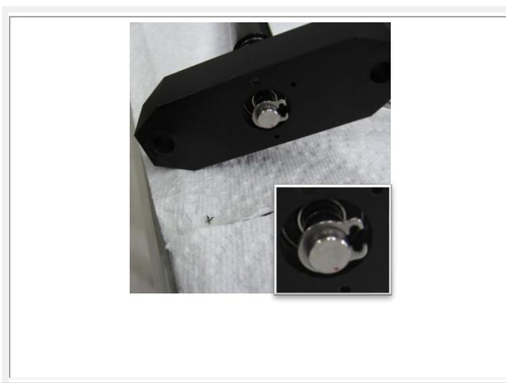
12. Install the E-Ring on the end of the shaft. Use Shim 9002061 as necessary to ensure a snug fit.
