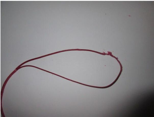
**Figure 42. Bad Loop splice, worn and torn**
