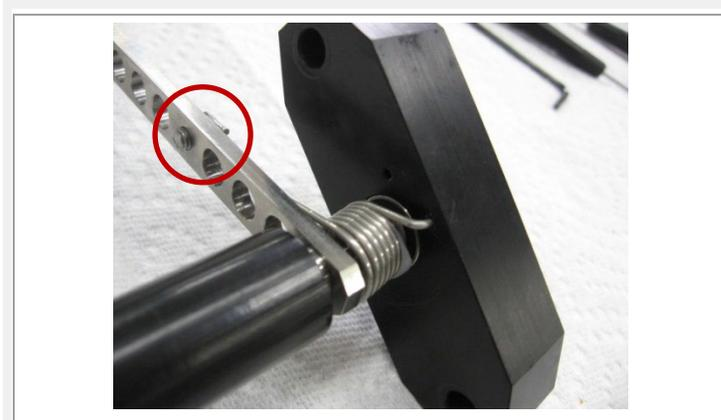
10. Install the new Spring on the shaft. Apply loctite 242 to the M4 screw (circled in red). Torque to 10.6 in-lbs.
