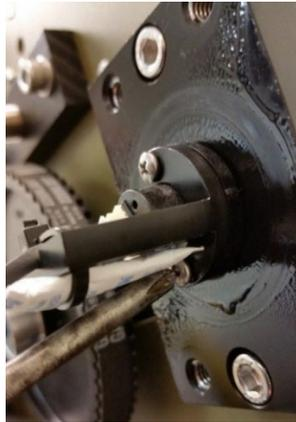
Remove one of the two Phillips head encoder alignment screws. Apply one drop of Loctite 425 to the threaded end. Reinstall the screw snugly, but loose enough to allow rotating the encoder. Repeat these steps for the second encoder alignment screw.
