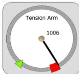
With the tension arm fully retracted, view the tension arm position on the RapidCAST software.
