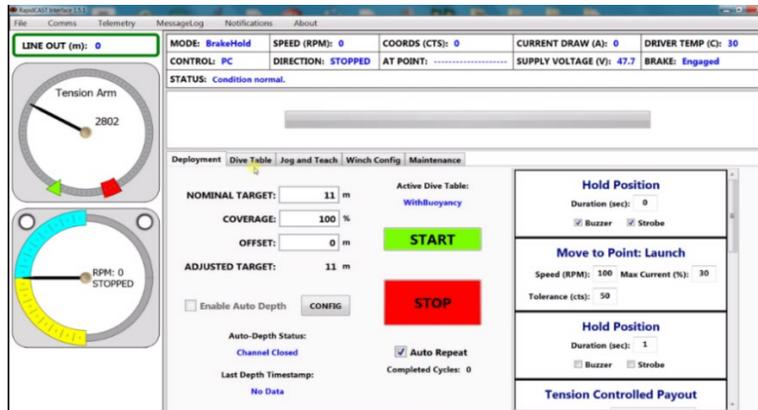
**Driver Temp:** Displays the temperature of the motor controller. This value will increase or decrease depending on the load applied to the motor. Note: Motor will shut down at 70C.
