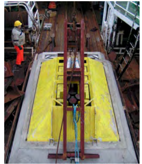
Figure 4. ADCPs were mostly deployed atop short moorings. At the shallowest site, the ADCP was put in a seabed frame to reduce the chances of being snagged by fishing trawlers. Photos: Hansen et al. (2015) Technical Report. See text
