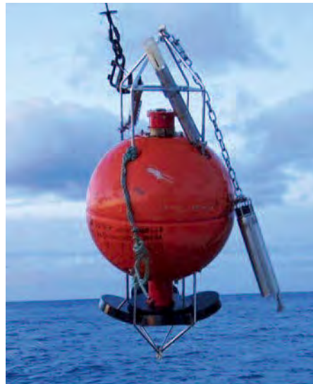
Figure 4. ADCPs were mostly deployed atop short moorings. At the shallowest site, the ADCP was put in a seabed frame to reduce the chances of being snagged by fishing trawlers. Photos: Hansen et al. (2015) Technical Report. See text
