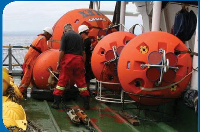
Teledyne RDI ADCPs mounted in top buoys of an ASCA mooring array.
