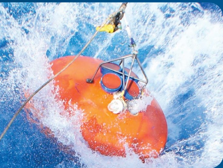
Long Ranger ADCP atop mooring for Agulhas System Climate Array (ASCA).
