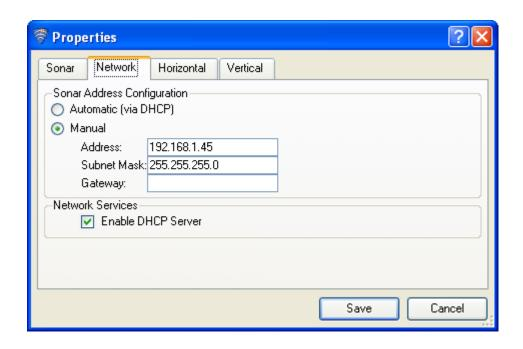
4. Reset the sonar by powering the sonar down for 10 seconds, then powering it back up. The sonar will now come up with the new IP address.
