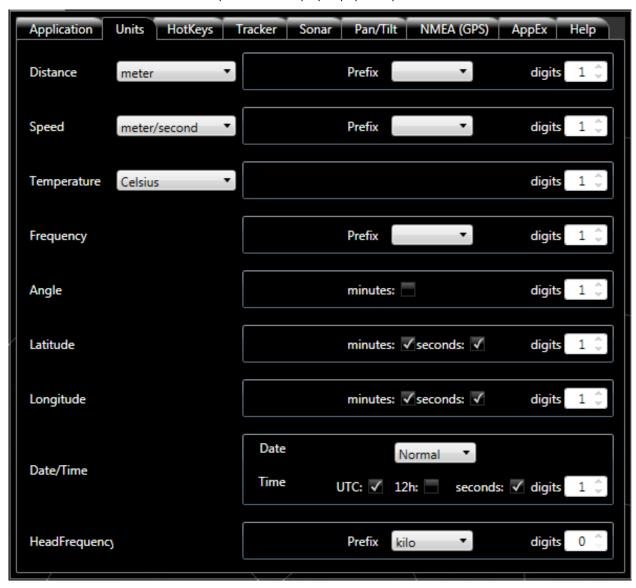
**DateTime:** This control allows you to change the format of the time displayed on the lower right hand corner of the ProViewer window. When data is recorded, the UTC time is always saved in the file, along with the time zone information. So UTC can be selected later for display, to give a definite time when the data was recorded, regardless of the time zone at that location.
