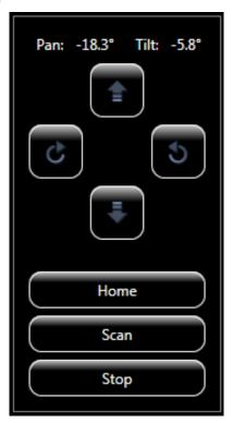
The arrow keys provide manual control, while the **Home**, **Scan**, and **Stop** button provide automatic control with settings as described in the previous section. The **Stop** button causes all automatic control (either **Scan** or **Home**) to cease immediately. The **Scan Speed** is applied to both the **Home** and **Scan** functions. Note that automatic control buttons are only visible for pan/tilt models that support these advanced functions.
