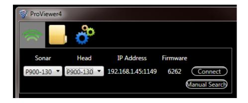
If no sonar head is discovered using ProViewer's auto-discover, click the **Manual Search** button, type **192.168.1.45** (the default Sonar IP address for all BlueView sonar systems), and click the **Try to Connect** button, as shown below:
