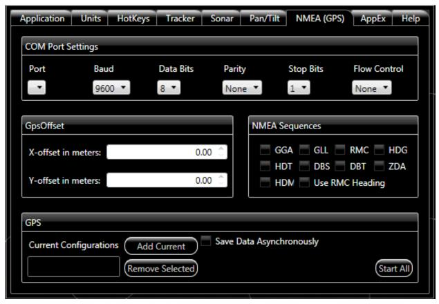
**COM Port Settings:** In this section, the proper COM port values corresponding to your GPS device must be filled in. The official NMEA setup is 4800 baud, 8 bits, no parity, one stop bit. Some newer devices use faster baud rates. Note that the current setup only supports a situation where all NMEA devices are consolidated to a single connection.
