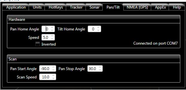
**Pan Home Angle:** Set the pan angle which will be returned to when the **Home** button is clicked on the pan and tilt controls.
