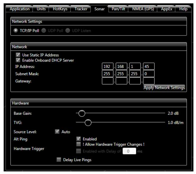
TCP/IP Poll: Sets up a direct connection between ProViewer and the Sonar over TCP. This is the standard configuration.
