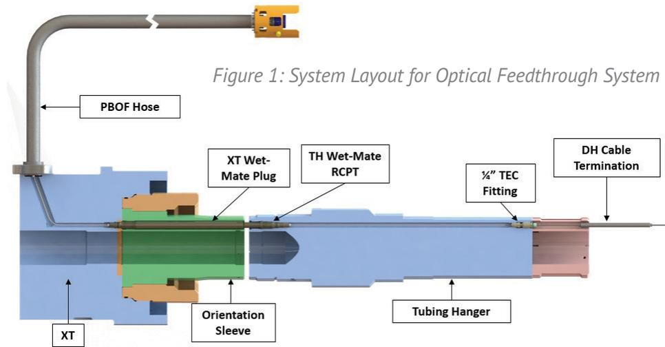
Figure 1: System Layout for Optical Feedthrough System
