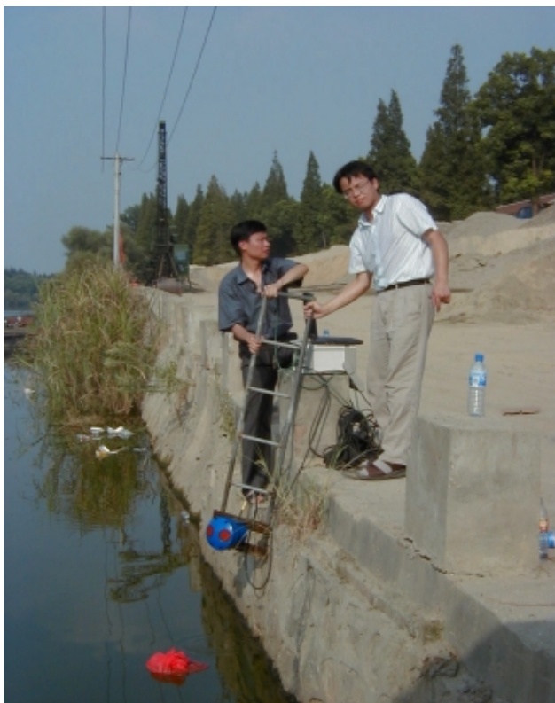
Figure 1: 1200 kHz ChannelMaster H-ADCP at the test site
