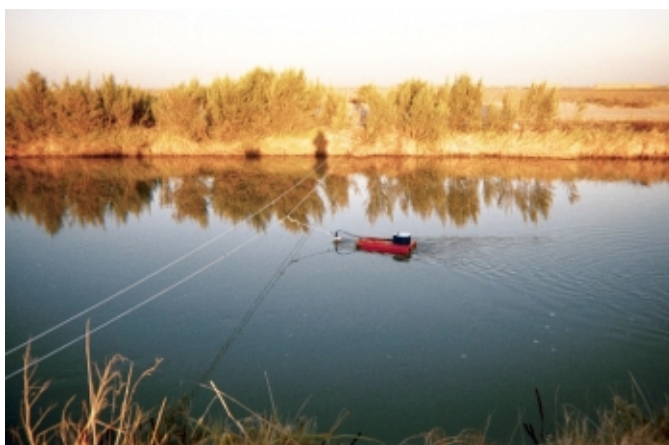
Figure 1: StreamPro attached to a pulley system at the test site.
