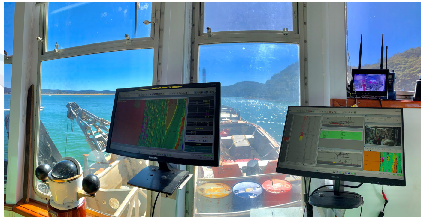
The Teledyne PDS Software is used to visualize and control the dredge progress in real time directly from the operators cab. Photo credit: McQuade Marine
