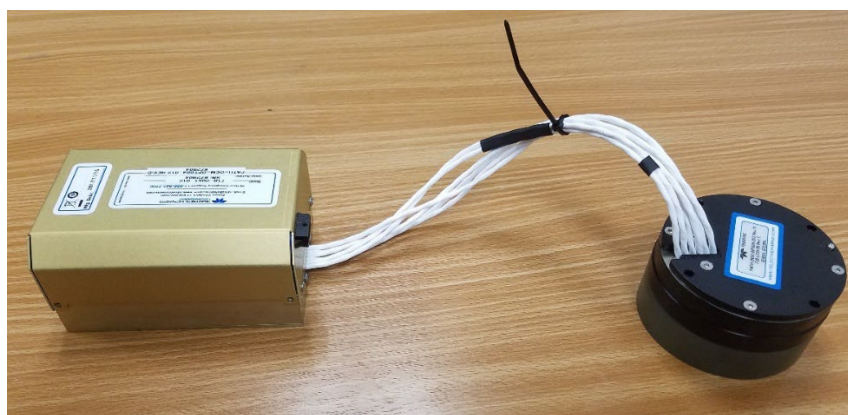
Figure 6. OEM 600kHz Pathfinder Transducer Connections
