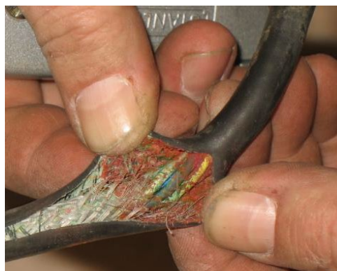
Figure 25. Do not use Zip-Ties Directly on Cables
