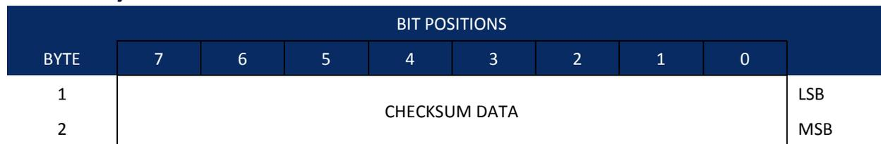
**Figure 25. Binary Checksum Data Format**
