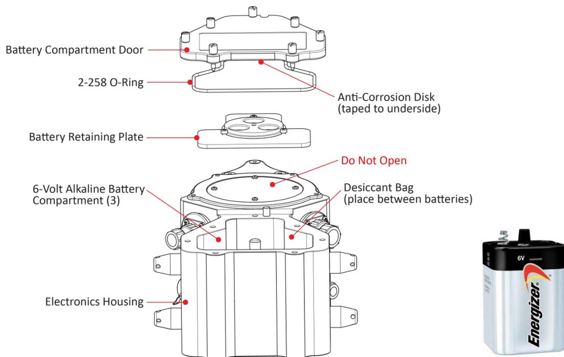
Figure 10. Battery Replacement
