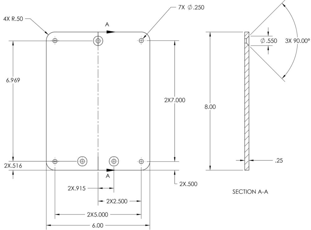
**Figure 29. Sensor Mounting Plate Dimensions**
