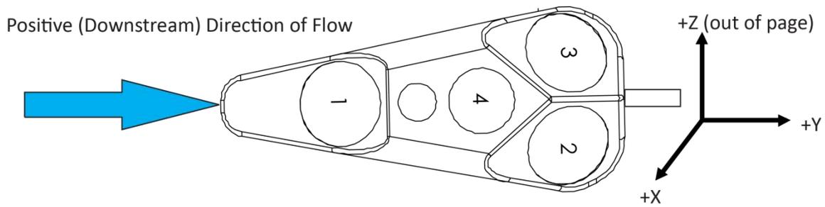
Figure 4. V-ADCP Instrument Coordinates
