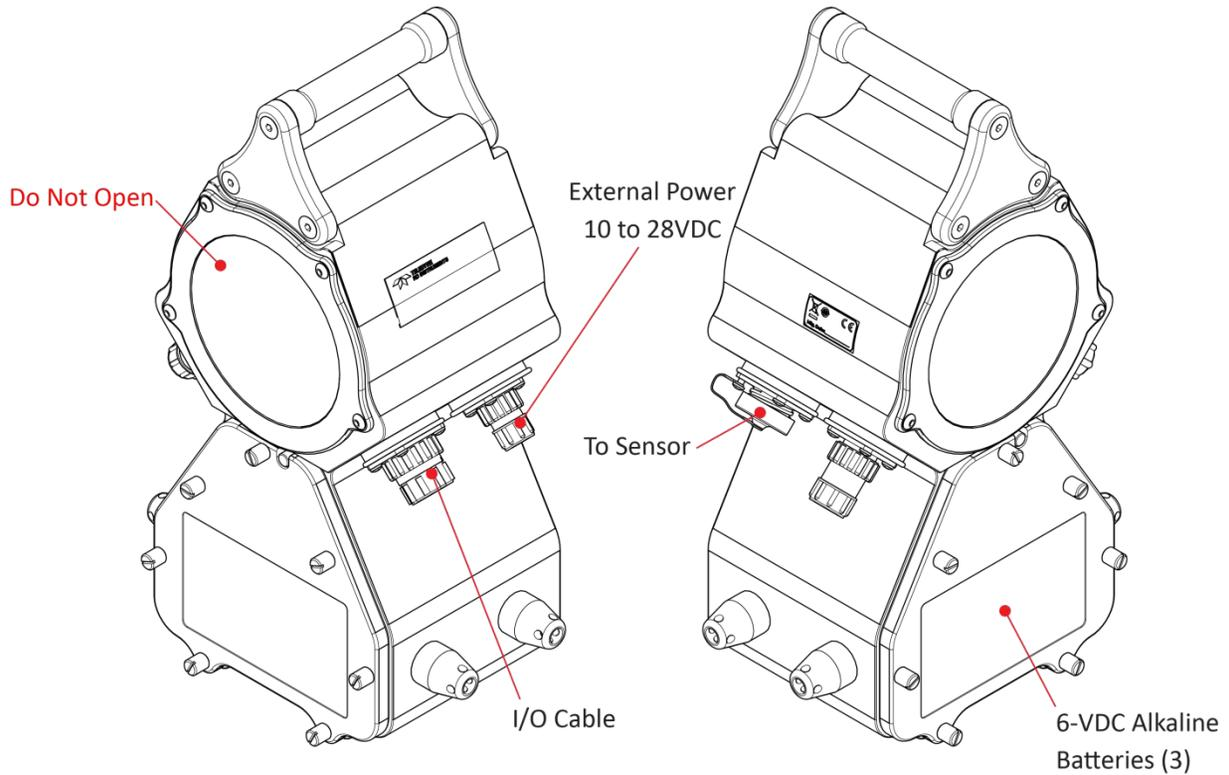
**Figure 2. V-ADCP Electronic Housing Overview**
