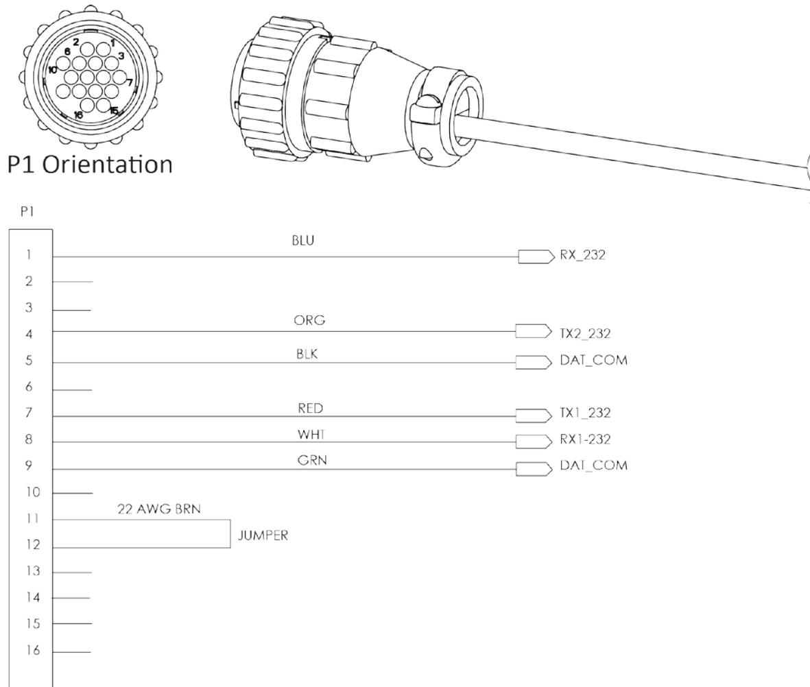
**Figure 8. I/O Pigtail Cable**
