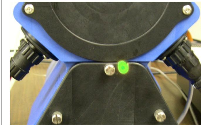
Disconnect the serial cable from the electronic housing and connect the dummy plug.
