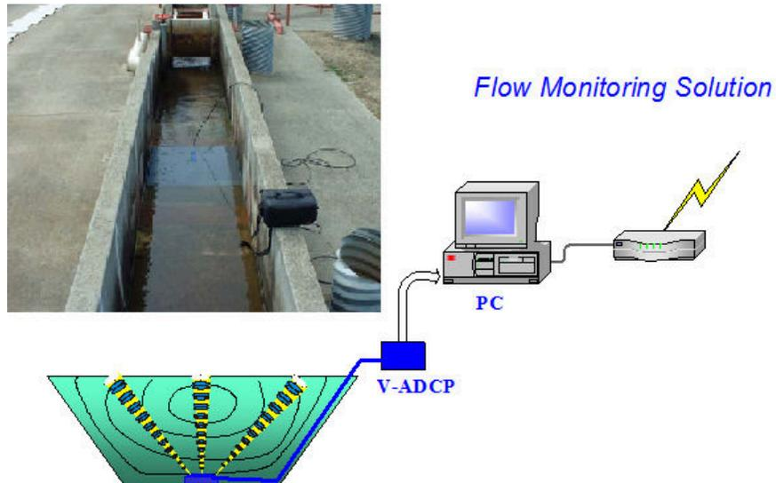
Figure 6. V-ADCP Installation Example
