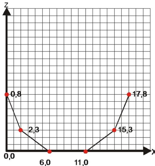
**Figure 12. Channel X – Z Pairs**
