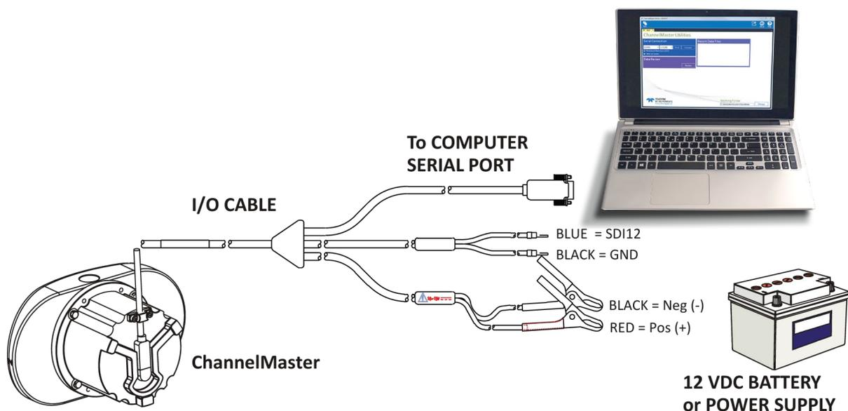
Figure 1. ChannelMaster Connections with SDI12
