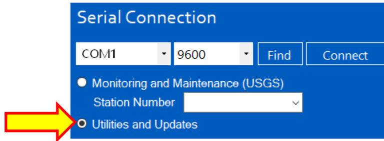
3. Enter the ChannelMaster's communication settings by selecting the **COM Port** the cable is connected to and **Baud Rate** from the drop-down lists.
