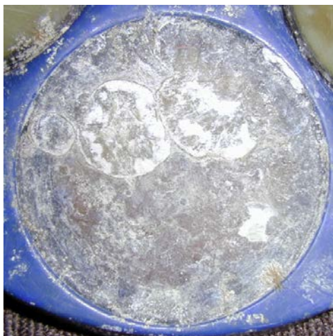
Figure 15. Barnacle Damage to Urethane Face
