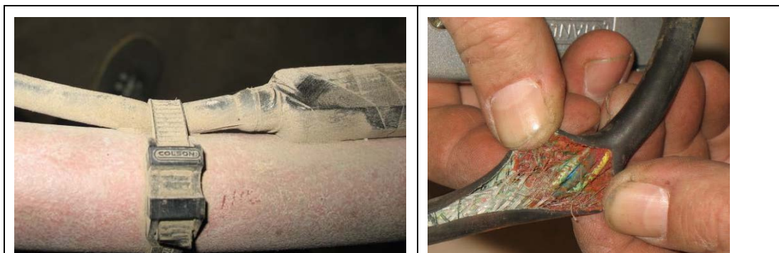
Figure 5. Do not use Zip-Ties Directly on Cables
