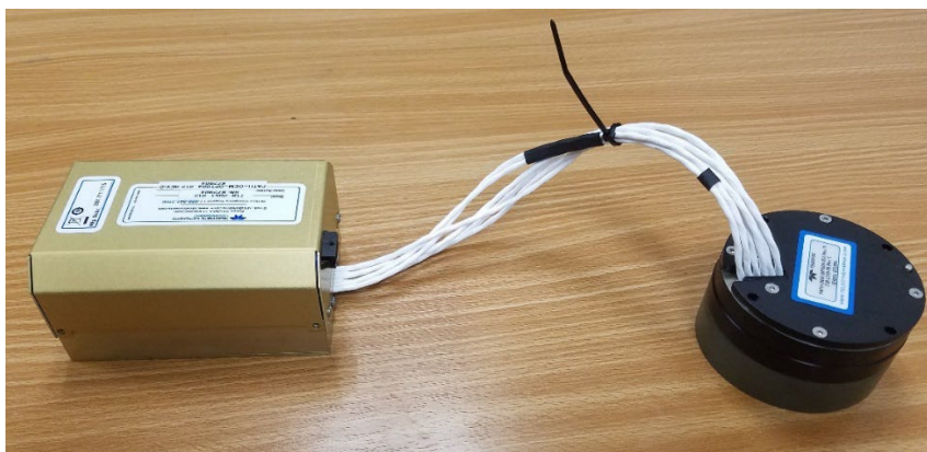
Figure 6. OEM 600kHz Pathfinder Transducer Connections
