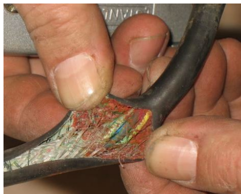
Figure 24. Do not use Zip-Ties Directly on Cables
