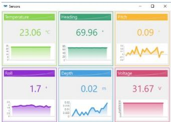
To verify the sensors are functional rotate and tilt the system and verify the Pitch and Roll sensor data is reasonable. Rotate the system clockwise and verify the heading increases. Validate the accuracy of beam 3 at 0, 90, and 180 degrees. If the heading is off by more than 2 degrees, calibrate the compass. If the pressure is not zero, zero the pressure sensor.
