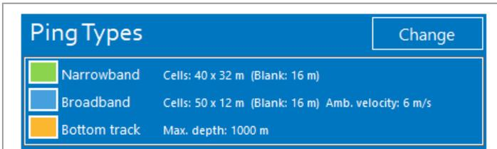
Check the **Ping Type** tab has **Narrowband**, **Broadband**, and **Bottom track** active.
