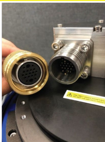
Figure 3. Connecting the Data/Power/Comm Underwater Cable
