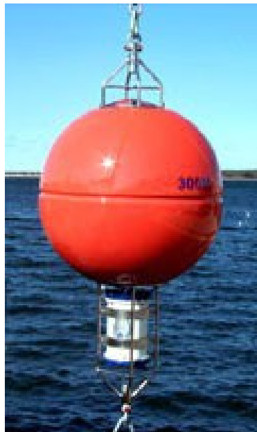
Figure 17. Buoy Mount with External Battery
