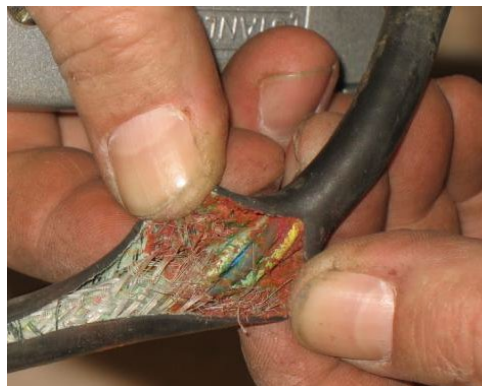
Figure 9. Do not use Zip-Ties Directly on Cables
