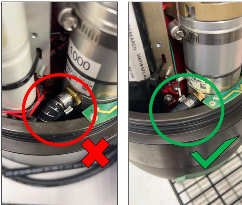
*Incorrect tubing (Left) is clear with silver spiral. Correct tubing (Right) is solid matte black.*
