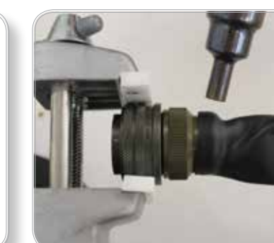
Heat shrinkable harness manufacturing
