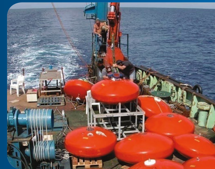
Low-drag flotation was installed on many LOCO moorings due to strong currents in Mozambique Channel.
