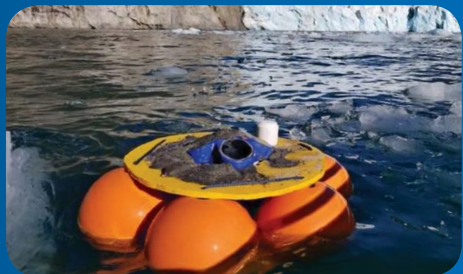
Sentinel V ADCP during recovery after being deployed for two weeks near LeConte Glacier.
