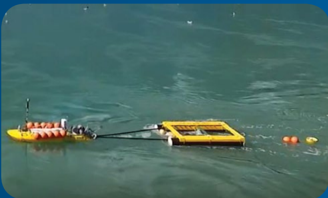
ADCP mooring was deployed using an unmanned raft towed by a ROSE vehicle (both designed/built by June Marion).
