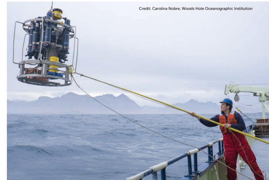
Deployment of Teledyne RDI ADCP with CTD package in station near the coast of Greenland on an OSNAP cruise in the North Atlantic. Teledyne floats and gliders contribute directly to understanding of climate change and impacts on the ocean.
