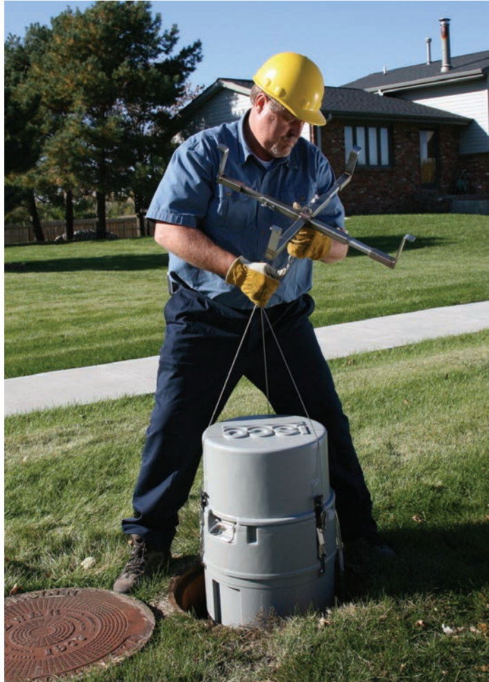
A Teledyne ISCO sampler is used in a neighborhood to collect wastewater samples for the detection of COVID-19.
