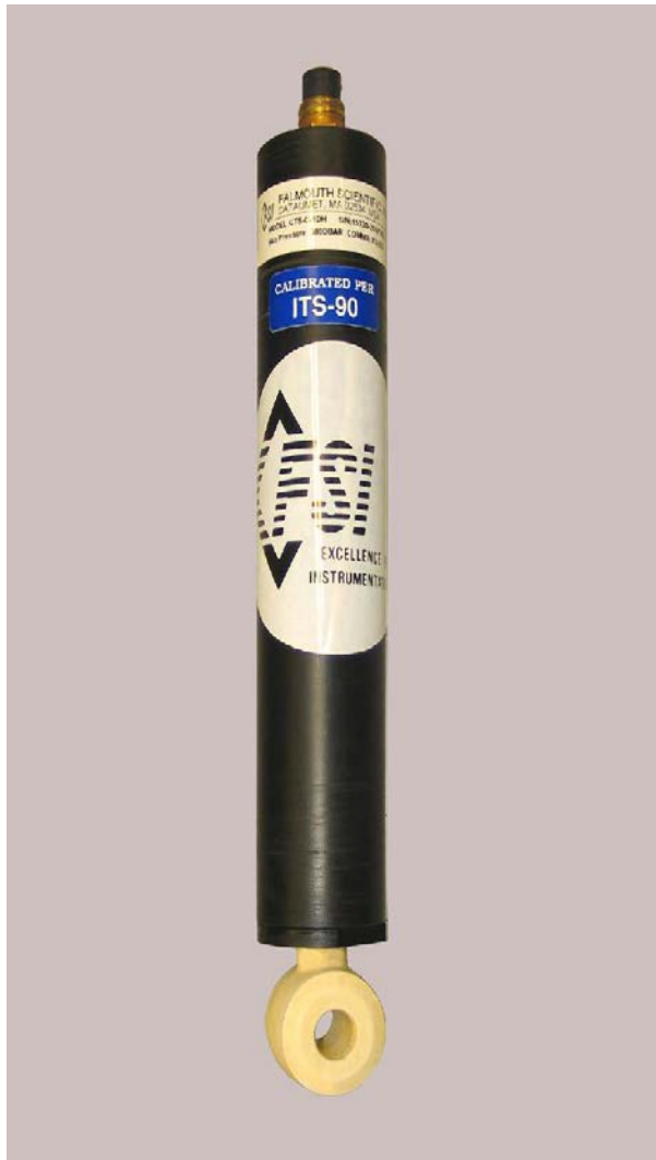
Figure 1. The 500-Meter Rated CT Sensor with Internal Temperature Sensor as a Completely Assembled Instrument
