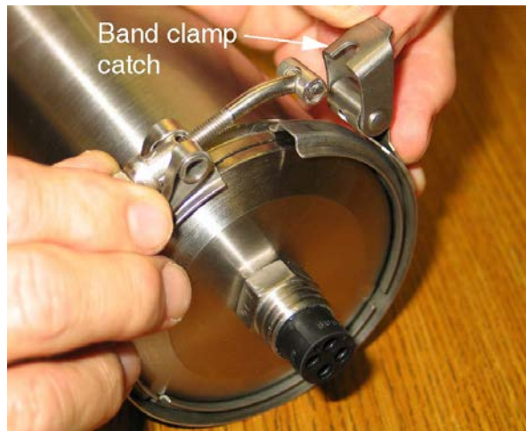
Releasing the Band Clamp Catch
