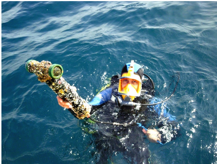
Figure 42. Cleaning the CTD-NH Sensor Head
