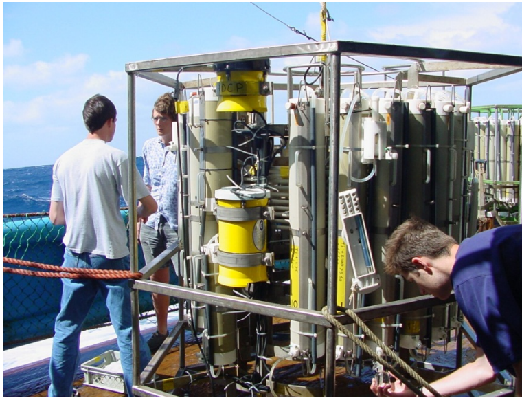
Figure 1. WorkHorse Monitors Mounted on a Rosette
