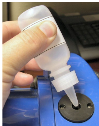
Figure 15. Filling the Pressure Sensor Cavity with Oil
