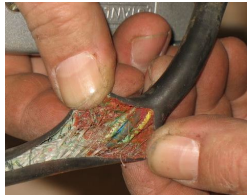
Figure 6. Do not use Zip-Ties Directly on Cables
