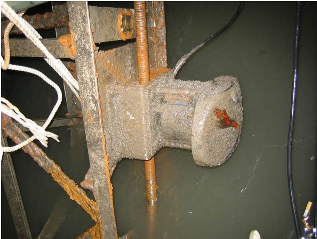
ChannelMaster 300 kHz after a three-month deployment. Photo by H. Huang
