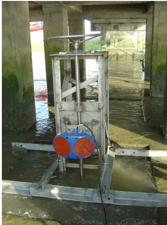
ChannelMaster 300 kHz located in Shanghai. Photo by H. Huang
