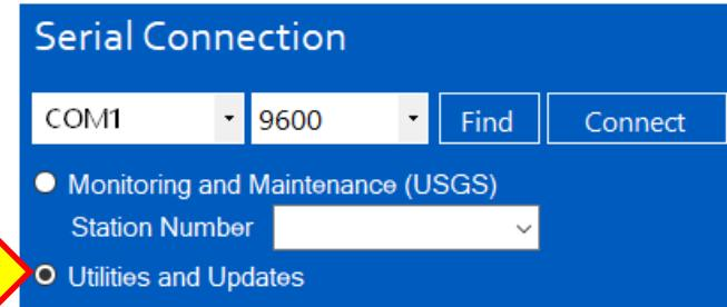
3. Enter the ChannelMaster's communication settings by selecting the **COM Port** the cable is connected to and **Baud Rate** from the drop-down lists.
