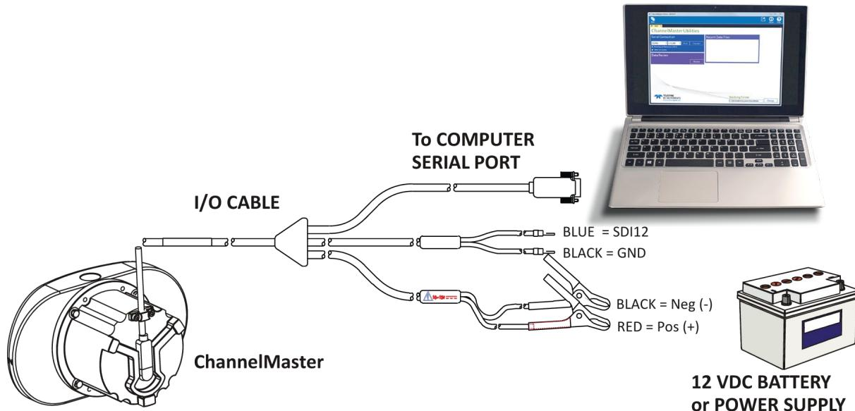
Figure 1. ChannelMaster Connections with SDI12
