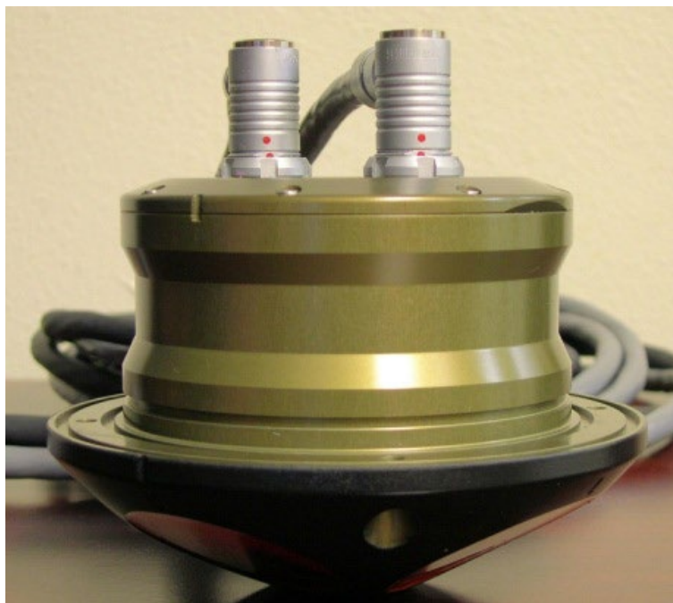
Figure 8. Transmit / Receive Cable Connectors
