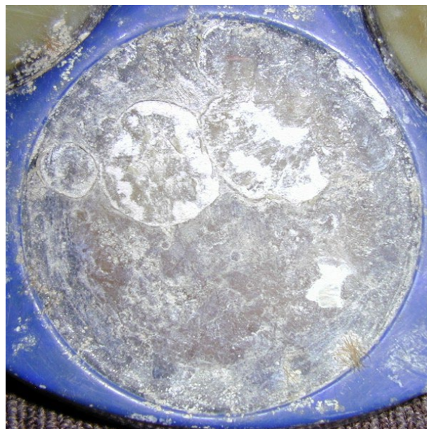
Figure 21. Barnacle Damage to a Urethane Face
