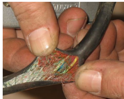
Figure 10. Do not use Zip-Ties Directly on Cables
