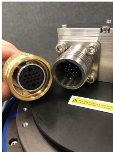
Figure 3. Connecting the Data/Power/Comm Underwater Cable
