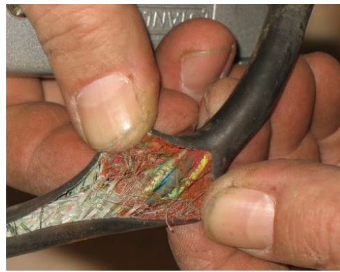
Figure 6. Do not use Zip-Ties Directly on Cables
