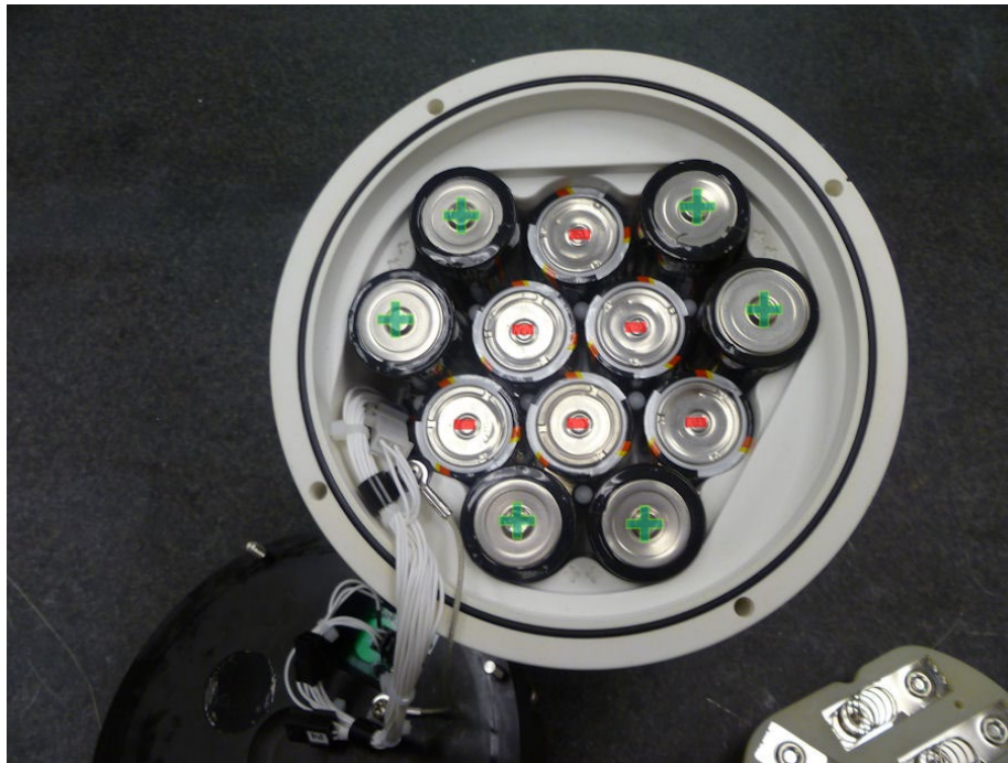
Figure 57. D cell Battery Replacement
