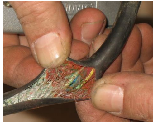
Figure 45. Do not use Zip-Ties Directly on Cables
