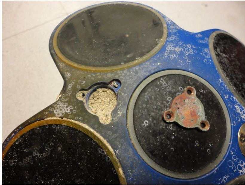
Figure 74. Pressure Sensor Cavity with Sand
