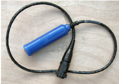
Figure 18. StreamPro Transducer Assembly and Cable Connector
