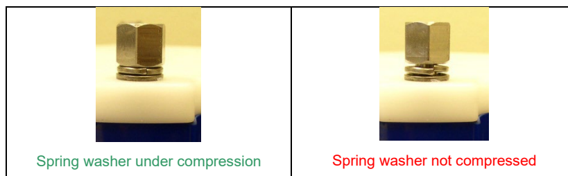
Figure 7. M6 Standoff Bolt on Electronic Housing Cover Plate
