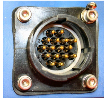
Figure 18. StreamPro Transducer Assembly and Cable Connector
