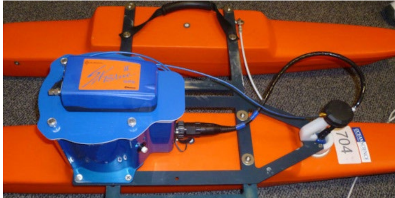
Figure 4. SXBlue II GPS/GNSS with Mounting Kit
