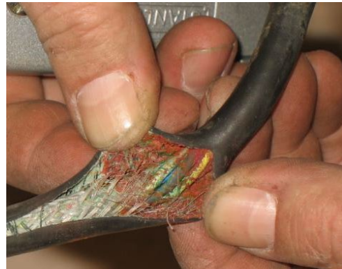
Figure 14. Do not use Zip-Ties Directly on Cables
