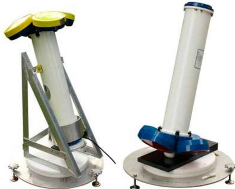
LR-1A is shown with Teledyne Long Ranger loaded for a UPWARD Profile Calibration
