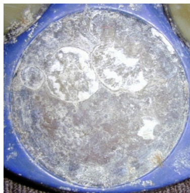
Figure 25. Barnacle Damage to Urethane Face
