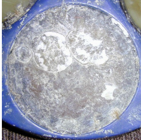
Figure 36. Barnacle Damage to Urethane Face
