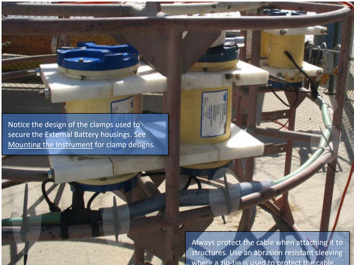
Figure 17. Cables Protected with Abrasion Resistant Sleeving
