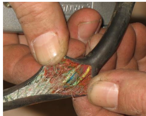
Figure 16. Do not use Zip-Ties Directly on Cables
