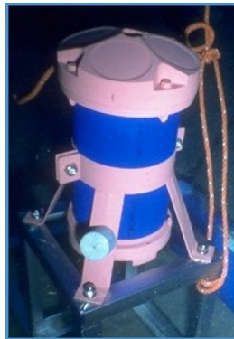
Figure 58. Antifouling Paint Applied to a WorkHorse Sentinel
