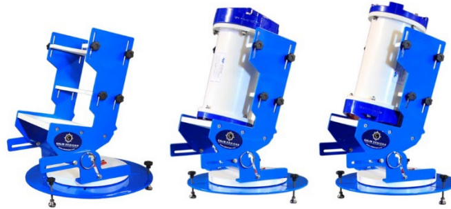
The WH-V is shown with a Teledyne RD Instruments Workhorse Sentinel ADCP loaded for UPWARD Profile Calibration (center) and loaded for a DOWNWARD Looking Profile Calibration (right).
